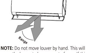
**NOTE:** Do not move louver by hand. This will cause the louver to become out of sync. If this occurs, turn off the unit and unplug it for a few seconds, then restart the unit. This will reset the louver.
