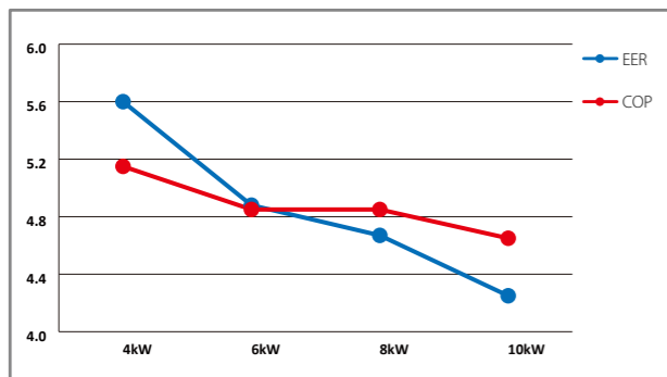
COP tested under: Ambient temp. 7°C/Outlet water temp. 35°C
