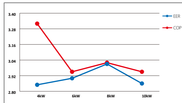
COP tested under: Ambient temp. 7°C/Outlet water temp. 55°C
